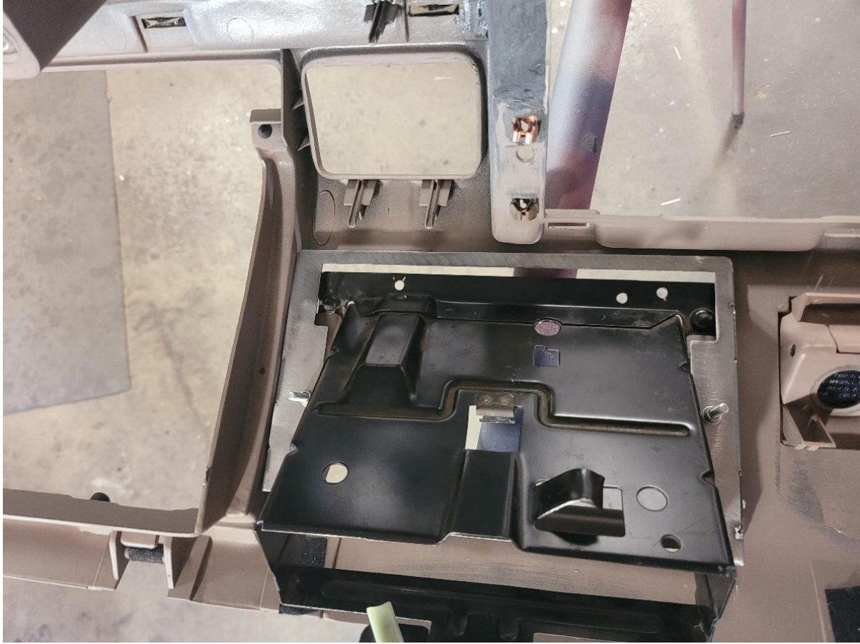
This is to give a reference to how the bracket is position is supposed to be from the back side
